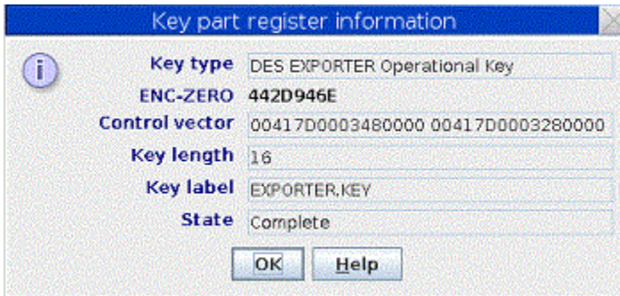
Figure 115: DES Key part register information - predefined EXPORTER key type in Complete state
